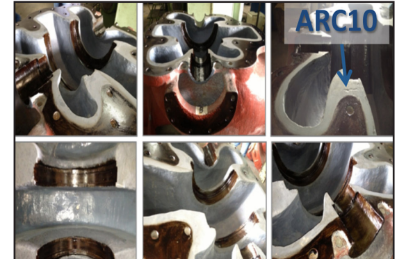
Reconstructed and finished pump
