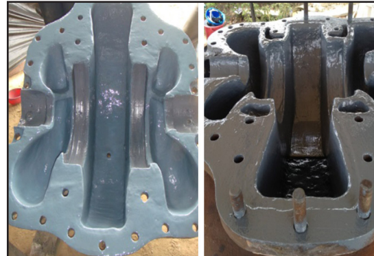
Repair being performed, body and cover
